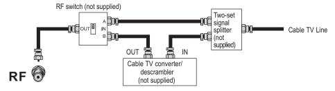
"A" position on the RF switch (not supplied): You can view all unscrambled channels by using the TV's channel keys.
